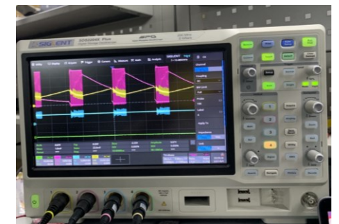
NCP1399A will easily enter burst mode when the loop design is poor
