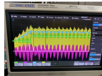
NCP 1616 PFC start-up process requires pull-up signal
